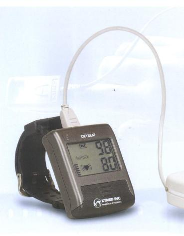
OXYBEAT is designed for long-term monitoring of patients. It is robust about motion artifact. This wrist-type pulse oximeter is adequate for sleep studies and for monitoring daily activities. With KTMED OxyView Software, data can be stored quickly and transferred by USB Port to a personal computer for data analysis.
